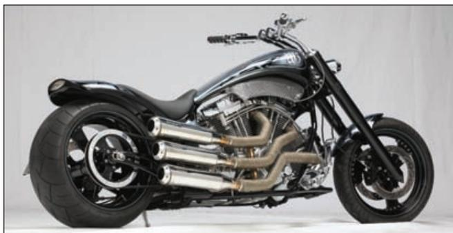
Probably less than 30 of the unique and powerful Feuling W-3 engines were produced before Jim Feuling died in 2002. Ruedi Steck was European importer for the engine. Sven Traber of Sven Cycles asked Peter Penzenstadler to build a custom frame for the triple that uses Twin Cam heads
