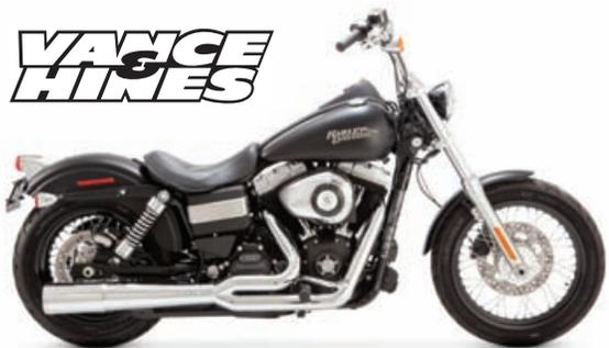
new 2012 pipes from the company, the Pro Pipe has the new flat plane mounting panel for the 12mm oxygen sensors. The Pro Pipe is finished with a CNC machined end cap and optional quiet and competition baffles are also available.
