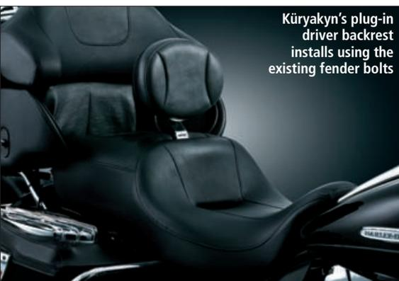
Küryakyn's plug-in driver backrest installs using the existing fender bolts
