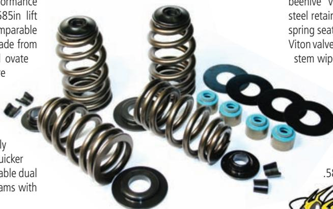
beehive valve springs, lightweight seven-degree steel retainers, machined heat-treated chrome moly spring seats, seat shims and valve locks and a set of Viton valve seals equipped with a spring loaded valve stem wiper system.
