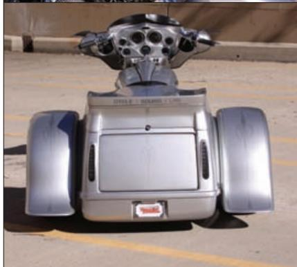
Trike fenders to cover the 20 x 10in wheels, a stretched tank kit, Original Trike Tour Pack, and the bottom of the trike's bodywork has been extended along its bottom edge.
