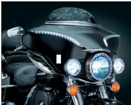
Phase 7 LED headlamps and passing lamps have impact resistant polycarbonate lenses
