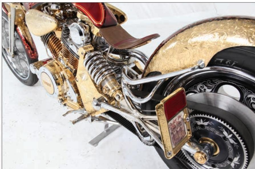
end of the bike. The Springer style fork used at the front was made from stainless steel legs with 6061 aluminum triple trees, with rake and trail both adjustable. At the rear end, the single-sided swingarm was built up from cold drawn mild steel and acts on a single offset shock absorber.
