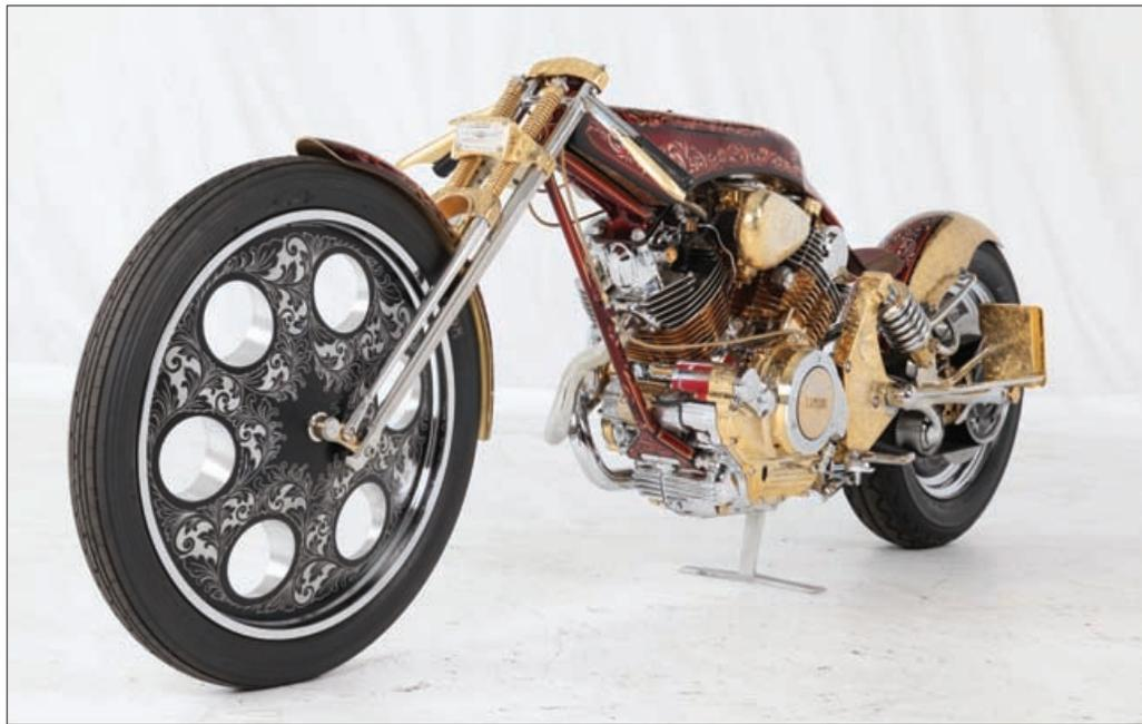
been shaped and welded together, while the front and rear fenders were hammered by hand into the shapes required to follow the profile of the tires. To finish the bodywork half of the fenders have been engraved and then gold plated, the same treatment being given to the underside of the gas tank, and then the rest has been painted. The red base coat with gold and silver leaf applied over the top was done partly by Stu Garland and partly by American motorcycle painter Horst.
