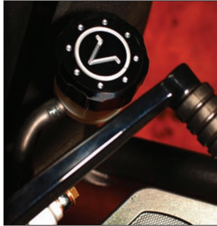
The master cylinder cap replaces the stock plastic item on '10 models and later Cross Roads and Cross Country models
