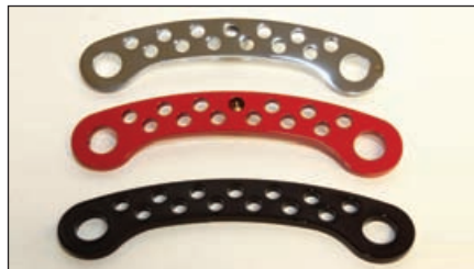
The lowering links for Victory bikes by Rick Fairless will reduce the ride height by 2in
