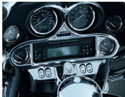
The brushed stainless steel rocker switch cover goes over the stock black switch cover
