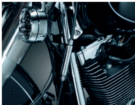
The chrome steel clutch cable adjuster cover from Kuryakyn replaces the stock rubber bellow
