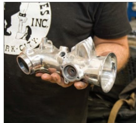
After 80 hours of work a combined one-piece manifold, throttle body and velocity stack for a Dyna project is still not finished
