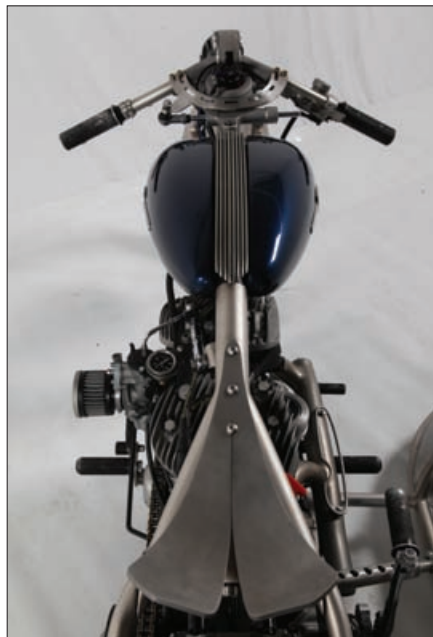
Laterally mounted steering damper on the handlebars helps to keep the bike under control when a passenger rides in the sidecar
