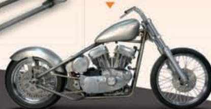
751472 NEW HARDTAIL FRAME for 2004 to present Sportster with 180 wide rear tire in 1 1/4" (32 mm) tubing, 30 degrees rake. Also available with 34 degrees rake. *(TÜV approval in progress)
