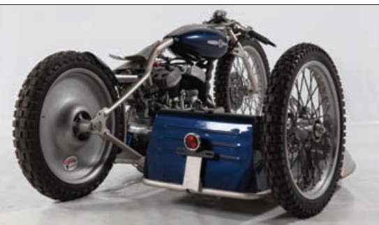
Gas tank at the rear of the sidecar offers an extended riding range
