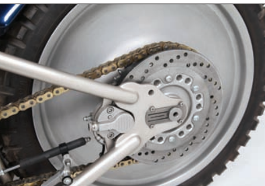
The brake disc mounted outside of the sprocket is gripped by a JayBrake calliper, just like those used on the front and sidecar wheels
