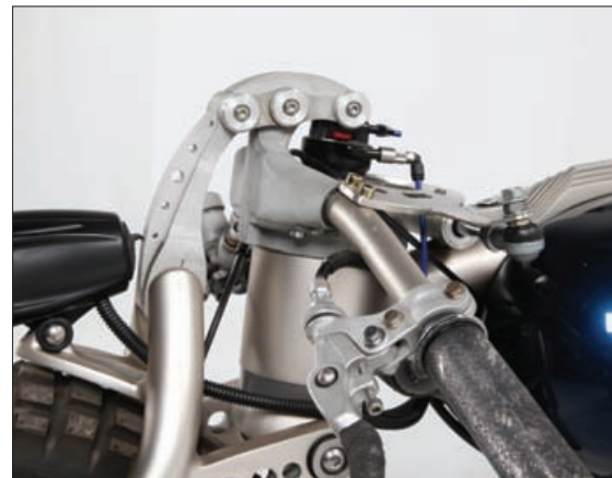
Described by builder Roman Bus as a 'Nivo' system, the air shock for the front suspension is inside the headstock
