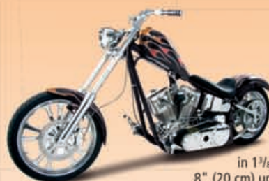
751472 NEW HARDTAIL FRAME for 2004 to present Sportster with 180 wide rear tire in 1 1/4" (32 mm) tubing, 30 degrees rake. Also available with 34 degrees rake. *(TÜV approval in progress)
