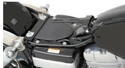
Drag Specialties has introduced its frame mount spring solo seat mount kit to make it easier to fit a solo seat to a bike
