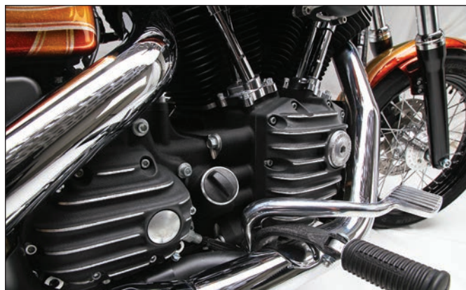
The Snatch cam and cable clutch covers from EMD can be used on Twin Cam applications
