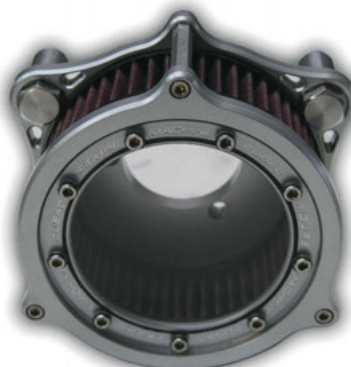
The Vision-5 for Sportsters uses a larger filter than the Vision-4
