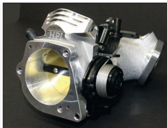
Delphi throttle bodies fit all cable driven Harley-Davidson motorcycles, and include the throttle body, manifold, throttle cable bracket, intake flanges and seals
