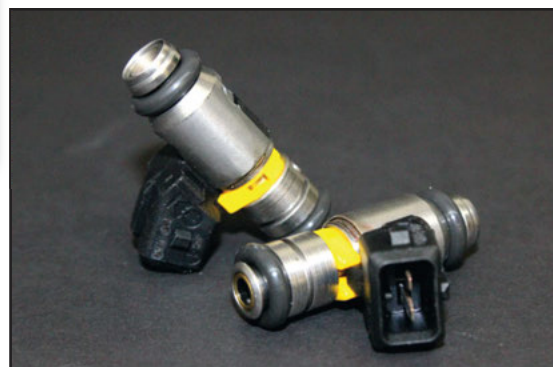
Yellow Band Injectors fit all '01-'05 cable driven motorcycles or '08-present throttle-by-wire, and provide a fuel delivery rate of 6.2gps (49.2lbs/h), which increases flow 43 percent over stock
