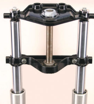
CUSTOM CYCLE ENGINEERING'S PINCH BOLT TOP PLATE FOR FLH
