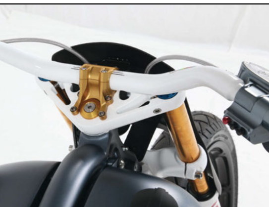
The handlebar clamp on HD 110 LE was sourced from Hope Technology and was originally intended to be used on a mountain bike
