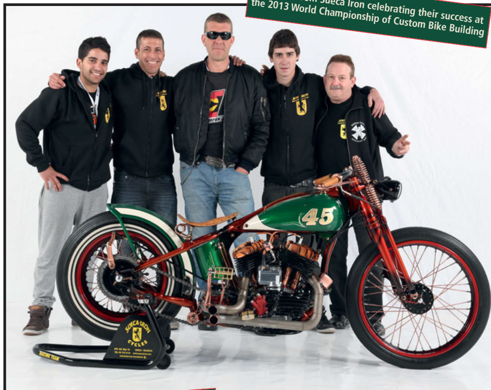
The Flathead motor was rebuilt relatively stock with the additions of a Joe Hunt magneto and one-off pipes
