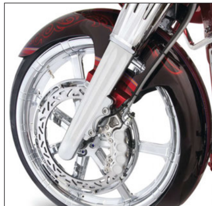
The Arlen Ness inboard brake kit includes an eight-piston caliper and is designed for use on 16in and larger Ness wheels
