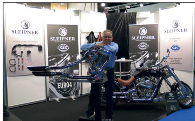
Lauge Jensen Engineering: Uffe Lauge Jensen chose INTERMOT for the debut of the EURO 4 compliant 'Sleipner' 1,800cc/111" 45 degree v-twin engine program co-developed with S&S Cycle. The EURO 4 emissions regulations come into effect in January 2016, and with a v-twin builder package that includes compliant catalytic converter equipped exhausts, this is the first aftermarket EURO 4 compliant engine available; www.sleipnermotors.com
