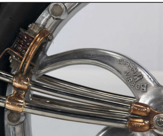
Magnets set in the rim of the front wheel provide the electricity to power the headlamps
