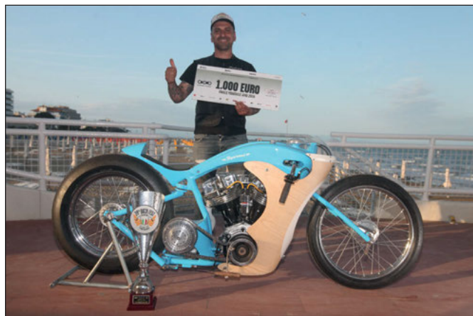
Apuania Choppers' "Flyin' Wood" features a hand made friction drive and rear wheel steering
