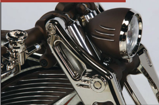
The unusual twin belt open primary was supplied by NH Power and features covers machined by Thunderbike
