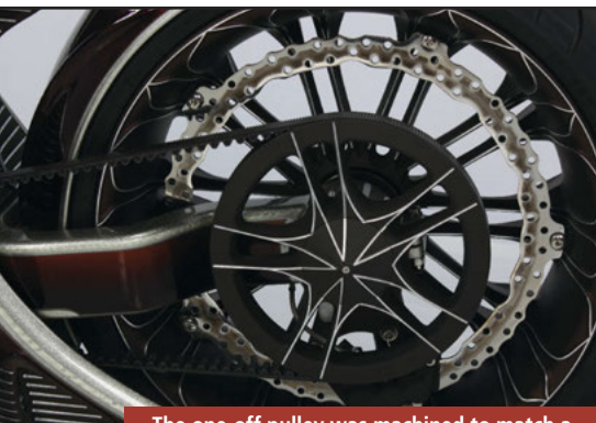
The one-off pulley was machined to match a 21in wheel, which was designed specifically for the build
