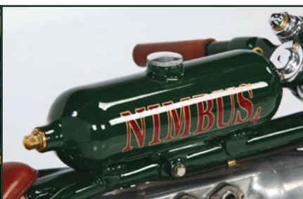
Tomas Tuner repurposed an old fire extinguisher as the gas tank for Nimbus
