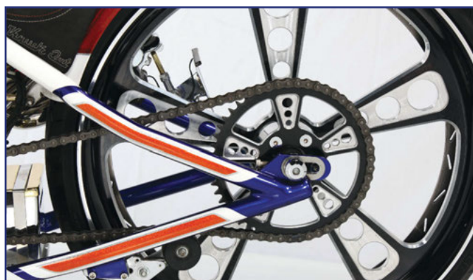
The 26in wheels from Southern Motorcycles are fitted with Riverside's own perimeter brake rotors to leave them as clean looking as possible
