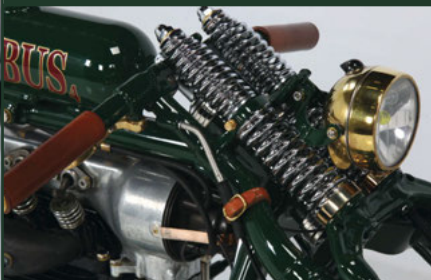
A 1920s Vitalux headlamp is used to give a period look to the front of the bike along with the use of a WLC Springer fork
