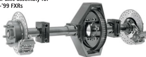
Rear axle assembly for '87-'99 FXRs
