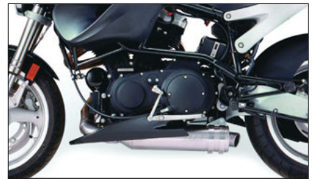
The SuperLight Stainless Series is a disc-based tunable slip-on muffler for Buell applications
