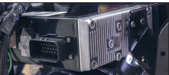
The HD1BT accepts the factory harness
