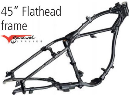
This reproduction 45" Flathead frame can be used as a stock replacement or as a basis to build a bobber or chopper from scratch. Dimensions and details exactly follow the factory counterpart.
