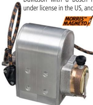
From the exterior you can hardly tell the difference from its historic counterpart, with cable activated, advance-retard, cotton braided spark plug wires and cast end plates, but inside it features various updates to make it even more reliable than the original, including an improved armature, coil and "modern" points. It is driven by the stock magneto gear, which is also available and mounts with 3/8"-16 bolts to the crankcase.
