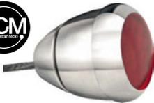
This shapely X-mini taillight features a billet stainless steel machined body, screw-on bezel and a detachable, studded rear section by which the TL-44 can sandwich any license plate or taillight bracket for an easy, self-supporting and clean installation. An acrylic lens with 3-wire (running/brake/ground) LED cluster provides full taillight function.
