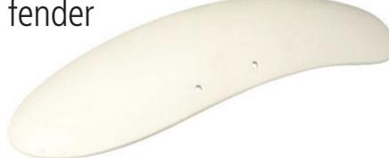
This front fender looks cut on both ends, for authentic original bobber styling. Pre-drilled for easy installation to the stock fender mounts. Made in Germany in GRP, it is primer coated for 16" tires and 3" rim width.
