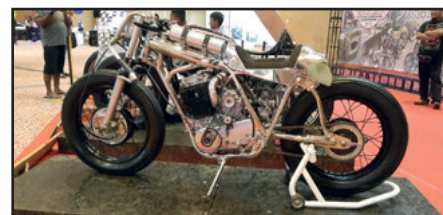
"Praying Mantis" by Beautiful Machines is a heavily modified and supercharged Yamaha SR400
