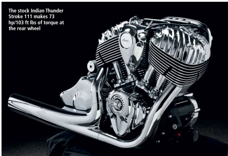
IPS is seeing gains of around 40 hp and claim around 112 hp and around 125 ft lbs torque - torque which rolls in at the bottom end with peak torque at around 3,800 rpm
