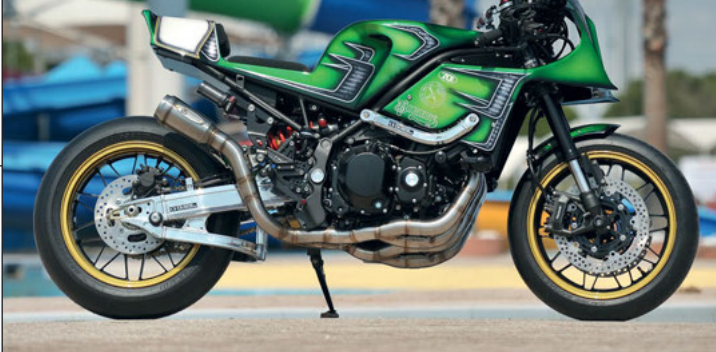
"Biker's Life Project" by Metal Dreams included extensive hand fabricated aluminum bodywork
