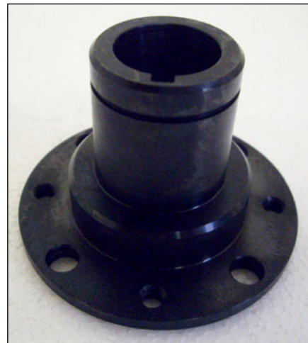
Steel inner drive hub, fits tapered main shaft Big Twins 1936-1984
