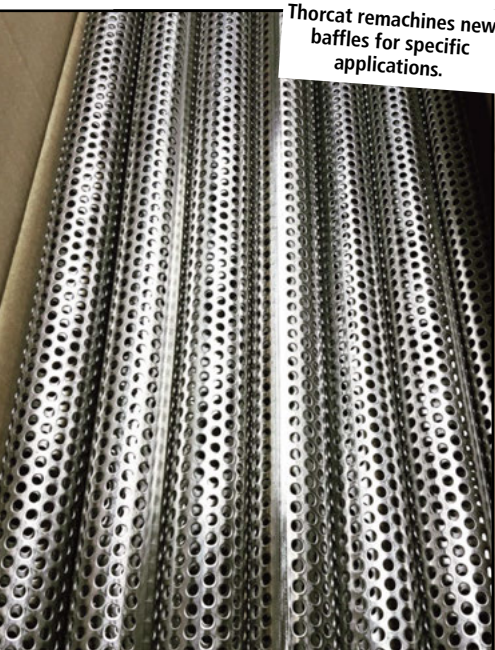
THORCAT produce its own baffle cores using Sanderson Machine Tools' exhaust core technology. Rather than making them perforated flat sheet, Malcolm Sanderson revolutionized the production and cutting of round cores, producing a better product faster and cheaper than anything else on the market at that time.
