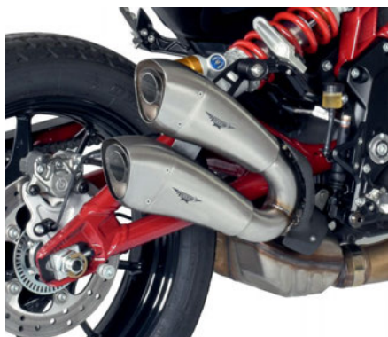
Hydroform Short for FTR 1200: available with or without dB killer. The craftsman-built 1 into 2 slip-on replaces the stock catalyst and has 25 hand TIG-welded pieces.
