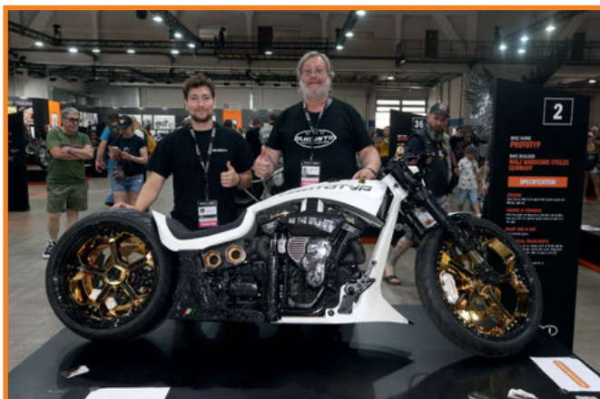
The "Public Choice" was a Walz/Augustin Motorcycles "Prototyp" Dragstyle Lowrider featuring lots of carbon and gold plating with a Rotrex centrifugal supercharged S&S engine motor.
