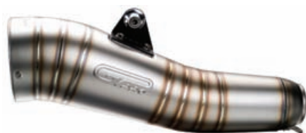
Nine sections of stainless steel are hand-welded together to create the GP Pro end can
