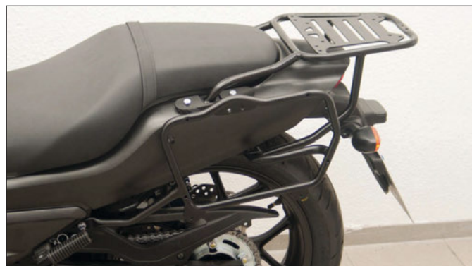
Fehling Flex system top and side case carriers for hard luggage from the likes of Givi, Kappa and others
