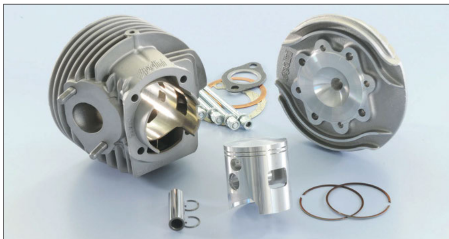
Polini's race-only Evolution-2 kit cast cylinder has a Nickel-Siliceous coated liner and gives Vespa's 125cc engine a 135cc displacement with stock 51mm stroke and 58mm bore. The gravity cast light alloy piston has two chromed cast iron rings; the head is a one-piece cast design with cooling fins
