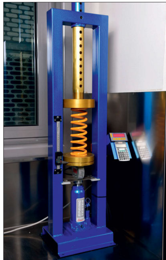
Andreani's electronic spring tester has been developed to accurately calculate spring rates
