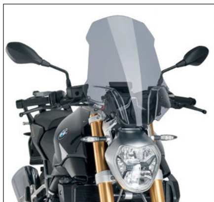
Virtual wind-tunnel tested acrylic touring screen
