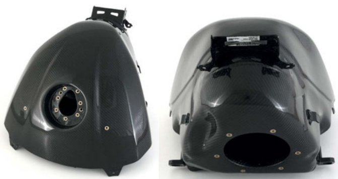
The FullSix monocoque fuel tank weighs in at just 1.8 kg, 75% less than the stock tank.
