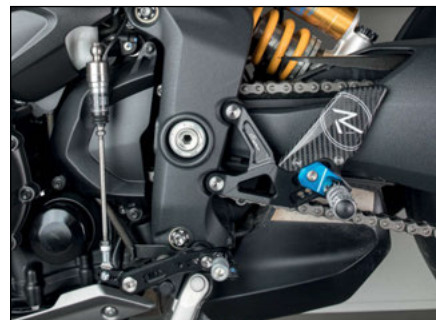
Speed Triple rearset, gear side
