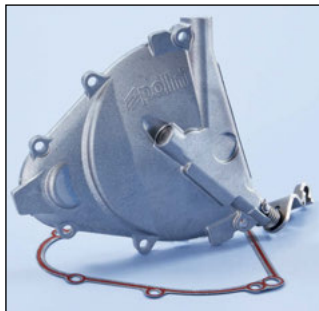
Vespa Special/Primavera/ET3 clutch case - interchangeable with the stock design, it has a rackwork pusher that allows fluid sliding with low friction coefficient. Suitable for standard and upgraded spring load clutches on race spec engines.
